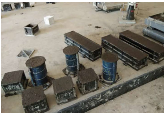
Fig. 6 Casting of specimens
