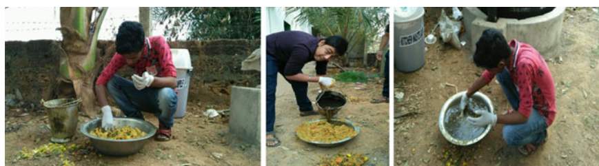
Fig. 1 Sample preparation of slurry from kitchen wastes
