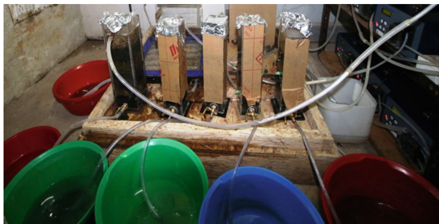
Fig. 1 Small-scale single-stage bioreactors engaged in nutrient removal
