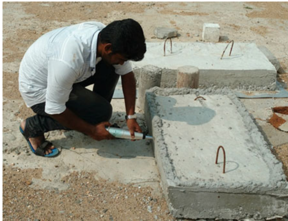
Fig. 3 Casted Conventional and Bubble deck slab
