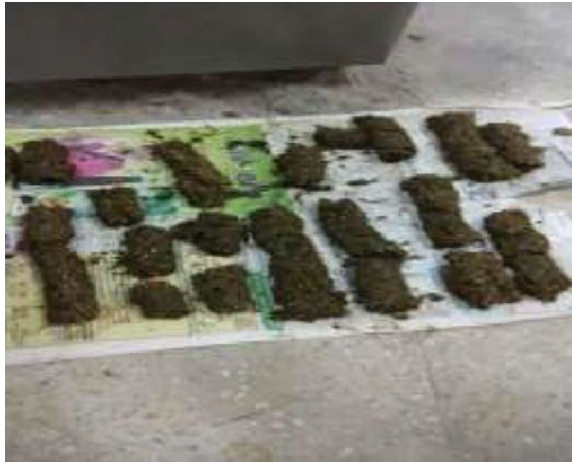
Fig. 4 Oven-dried briquettes of sample 1
