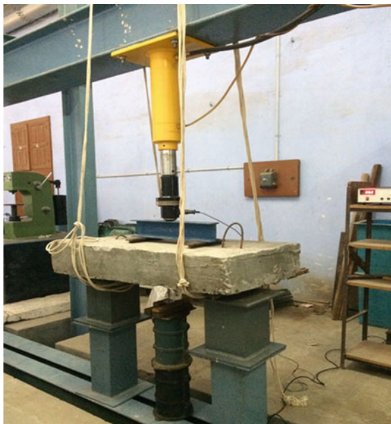
Fig. 4 Experimental setup of the slab
