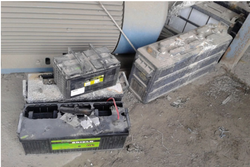
Fig. 4 Unsafe storage of scrap batteries
