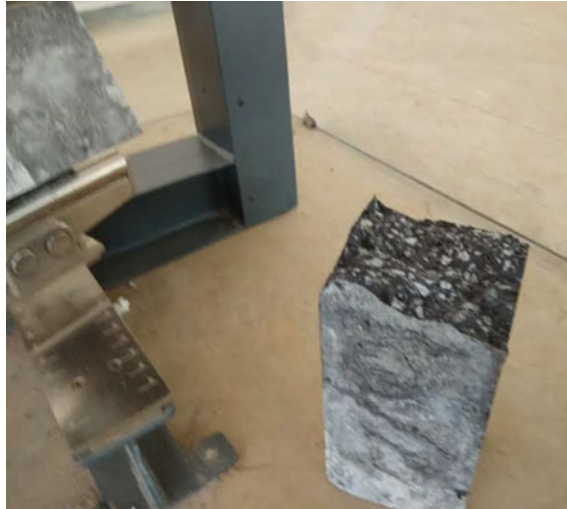
Fig. 10 Failure of flexure beam
