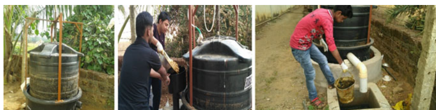
Fig. 2 Biogas plant set up for experiment
